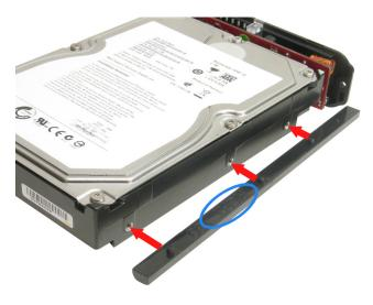
The picture below shows how the guide being attached to the hard drive correctly. If the guides are not properly installed, the hard drive cannot be inserted into the enclosure case.
